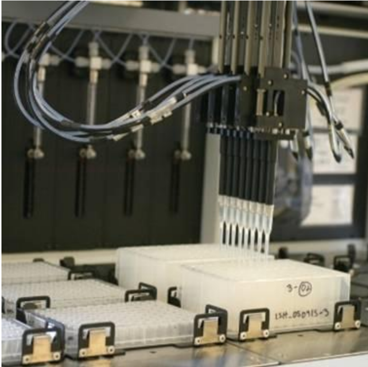
Figure 5. A Perkin Elmer Multiprobe II instrument was used for initial normalization of IVT reaction products to 30 ng/ \mu l with THE, aliquotting hybridization mix at 400 \mu l per well to ISH probe plates and final addition of 4 \mu l (30 ng/ \mu l) probe to ISH probe plates.
