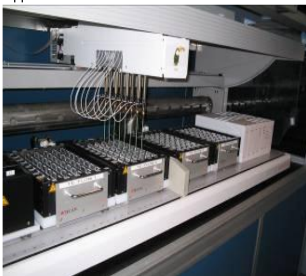
Figure 12. Customized Tecan robots were used to pipette solutions onto slides at programmed intervals, allowing the majority of the ISH procedure to be performed in an automated fashion (left). The “gripper” of a Leica CV5030 instrument automatically applied a coverslip to specimen slides (right).
