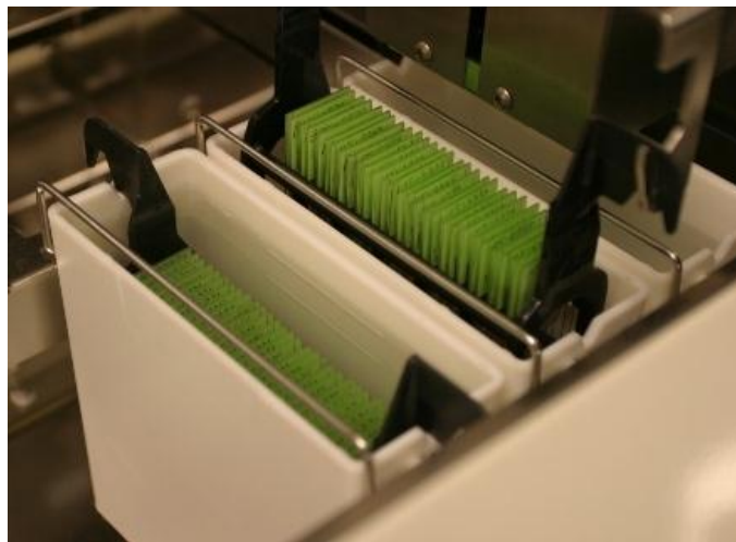
Figure 10. Leica Autostainer XL was used for the fixation and dehydration tasks. Acetylation is performed manually.
